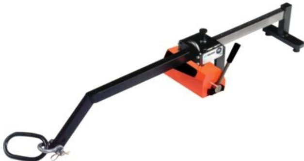
The Neo HV lifting arm, in connection with a Neo lifting magnet, is a versatile aid for handling loads from the horizontal to the vertical position and vice versa. For example, if a plate is on a pallet and you need to move it to a lathe, you must usually make use of chains, clamps, and at least two workers. With a lifting arm equipped with a Neo permanent lifting magnet, you will save manpower and make the operation more efficient.
