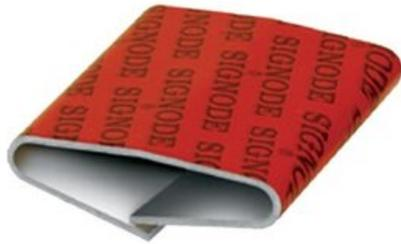
Ideal for round or irregular shaped bundles, push-type seals are used with a push-type tensioner to secure steel strapping. The flanges on a push-type seal completely overlap so both strap ends must be manually pre-threaded through the push seal before tensioning. These seals are usually crowned to prevent them from migrating too far into the hand tool during tensioning. A reverse notch joint is typically used to secure push-type seals.
