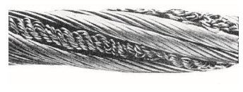
8. Protrusion of steel core resulting from shock loading.
