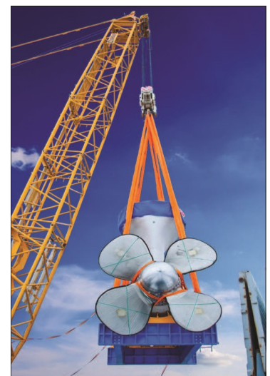
Lifting of a 305 t Azipod unit with Haklift 100 t roundslings.
