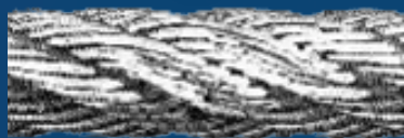
Local wear from contact with steel and vibration between the drum and the pulley.
