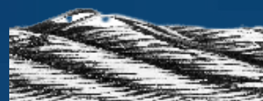
Exposed steel core due to transverse loading.
