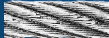
Wire wear and fractures caused by an excessively wide groove or small sheaves.
