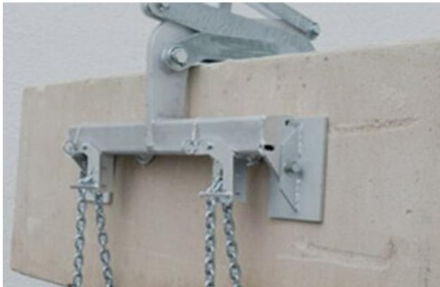
The galvanized wall panel lifting gear is used for the laying of horizontally positioned AAC wall panels. The profiled clamps ensure a high grip. If the safety chain is applied a transport high above the ground is permitted. The safety chain can be released by a tension rope of 10 m length.
